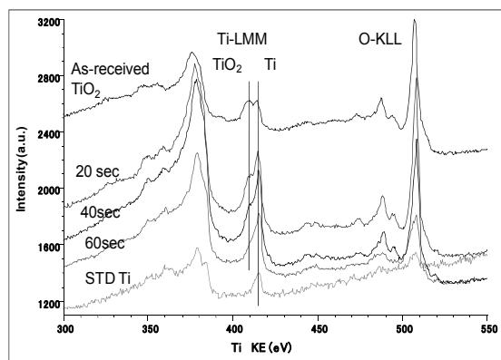
Fig. 2.  $\text{TiO}_2$  Auger spectra of as-received and after 20, 40 and 60 s sputtering by the 3 keV  $\text{Ar}^+$  ion. STD Ti is the standard spectra of metallic Ti.
