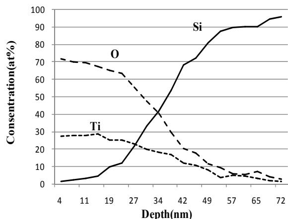
Fig. 6. AES crater edge profile for 30nm TiO<sub>2</sub> on Si etched by 1 keV Ar<sup>+</sup> ion.
