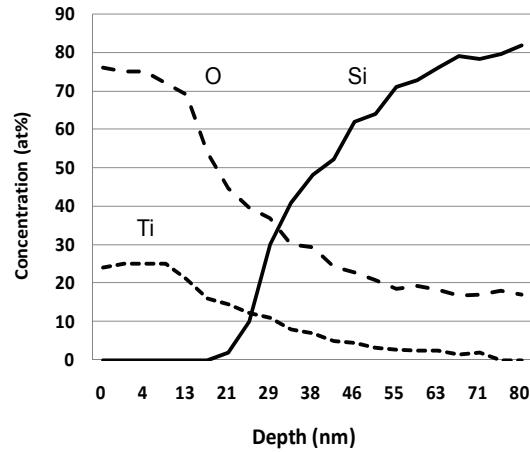
Fig. 8. AES crater edge profile for  $\text{TiO}_2$ (30nm) on Si(100) etched by EDI.
