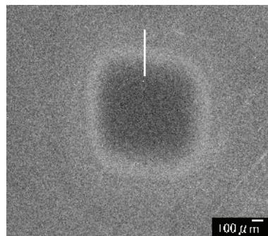
Fig. 5. SEM image of crater formed for TiO<sub>2</sub>(30nm) on Si(100) etched by 1keV Ar<sup>+</sup> ion sputtering. White line is the position of Auger 26 multi-points analysis.
