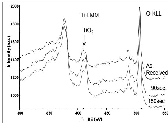
Fig. 3. TiO<sub>2</sub> Auger spectra of as-received and after 90 and 150 s sputtering by the 1 keV Ar<sup>+</sup> ion sputtering.
