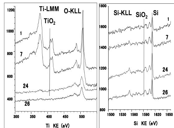
Fig. 9. Auger spectra from 26 multi-point analysis on the crater edge etched by EDI. The 1 point position is the spectrum at the top surface and the 26 is the spectrum at the bottom of the crater etched shown in Fig. 7.
