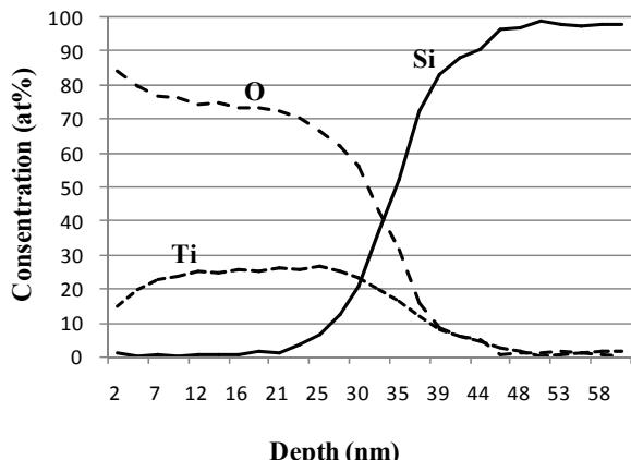
Fig. 4. Depth profile of TiO<sub>2</sub>(30nm) on Si(100) etched by 1 keV Ar<sup>+</sup> ion.
