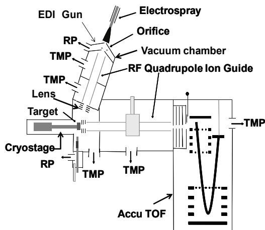
Fig. 1. Schematic diagram of the time-of-flight mass spectrometer equipped with an EDI Gun.
