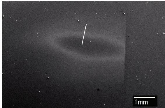
Fig. 7. SEM image of crater for  $\text{TiO}_2$ (30nm) on Si(100) etched by EDI. White line is the position of Auger 26 multi-points analysis.
